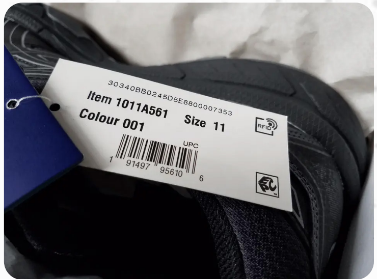
Example of an EPC label with an RFID tag built inside
